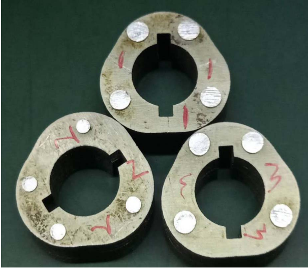
Fig. 5. Prototype of the VR resolver rotor optimized.
