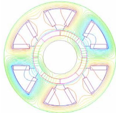
Fig. 12 FEM result: The magnetic field produced by the drive current in the motor shown in Fig. 4
