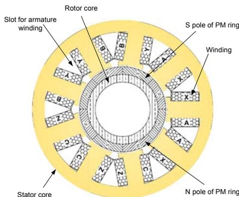
**Fig. 1** the PM-BLDC motor with surface mounted magnet on the rotor
