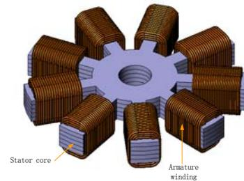
**Fig. 2** the fractional concentrated windings in spindle motor
