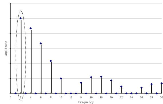
Fig. 8 The spectrum of the MMF generated by one phase current of the 2<sup>nd</sup> kind of winding
