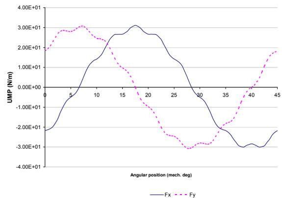
Fig. 13 The UMP generated in the 9-slot/4-pp spindle motor without drive current
