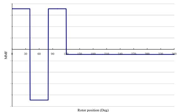
Fig. 14 The MMF generated by the one phase current of the 2<sup>nd</sup> kind of winding
