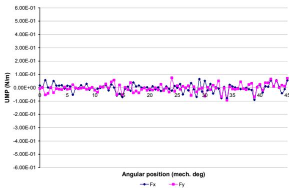
Fig. 10 FEM result: UMP of the motor shown in Fig. 4
