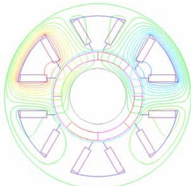
Fig. 11 FEM result: The magnetic field produced by the drive current in the motor shown in Fig. 3
