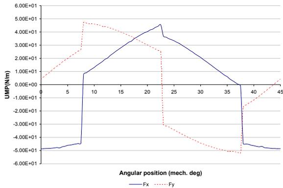
Fig. 9 FEM result: UMP of the motor shown in Fig. 3
