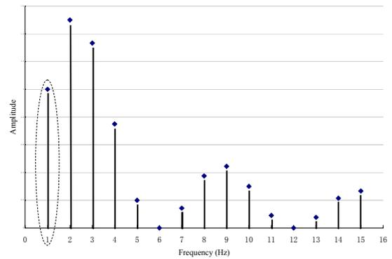
Fig. 7 The spectrum of the MMF generated by one phase current of the 1<sup>st</sup> kind of winding
