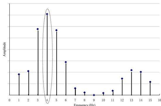
Fig. 15 The spectrum of the MMF generated by one phase winding of the 9-slot/4-pole spindle motor
