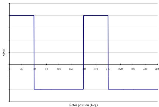
Fig. 6 The MMF generated by the one phase current of the 2<sup>nd</sup> winding
