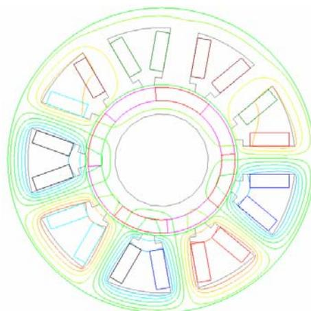
Fig. 17 The magnetic field produced by the drive current of the 9-slot/4-pole spindle motor
