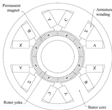
Fig. 4 The 2<sup>nd</sup> winding in the spindle motor with 6-slot and 4 pole-pairs
