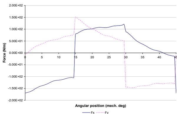
Fig. 16 The UMP generated in the 9-slot/4-pole spindle motor
