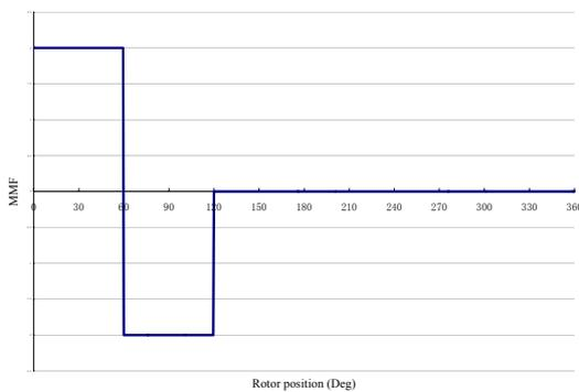
Fig. 5 The MMF generated by one phase current of the 1<sup>st</sup> kind of winding
