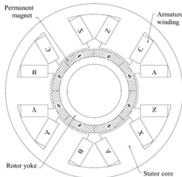
Fig. 3 The 1<sup>st</sup> winding in the spindle motor with 6-slot and 4 pole-pairs
