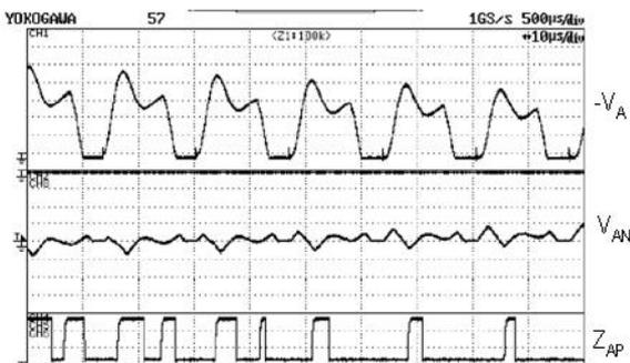
Fig. 12. ZCP level signal of phase *A* during silent period.
