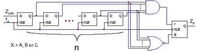
Fig. 13. Noise pulse filter with a set maximum noise width.
