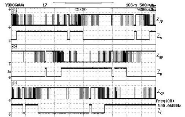
Fig. 15. Phase voltage ZCP signals with PWM chopping noises.
