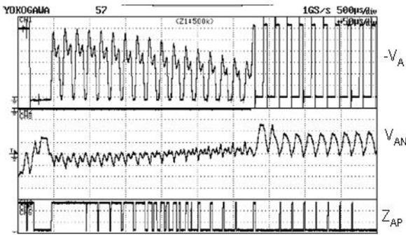
Fig. 11. Zooming in the phase voltage noises by PWM chopping.
