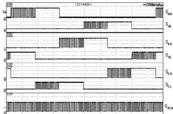
Fig. 7. MOSFET control signals for the inverter switches under alternate chopping control.
