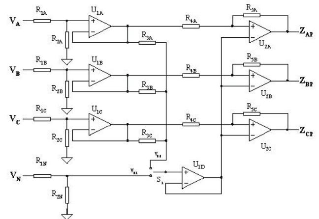
Fig. 9. Phase voltages and their ZCP detecting circuit
