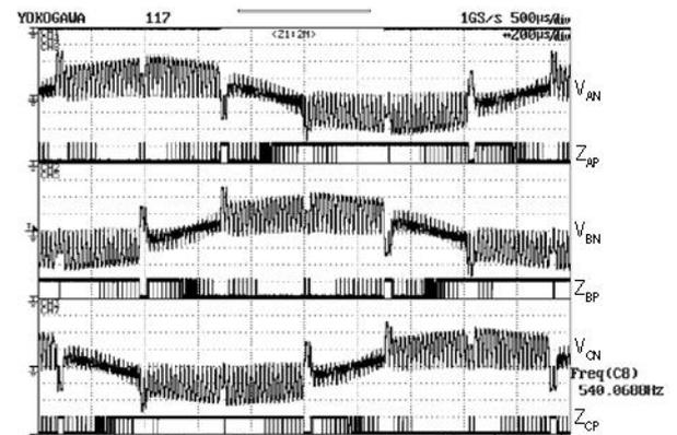
Fig. 10. Phase voltages and their ZCP level signals.
