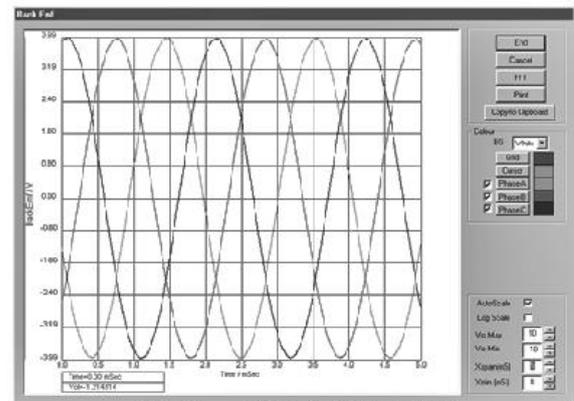
(a) Sinusoidal back EMFs at 7,200 rpm
