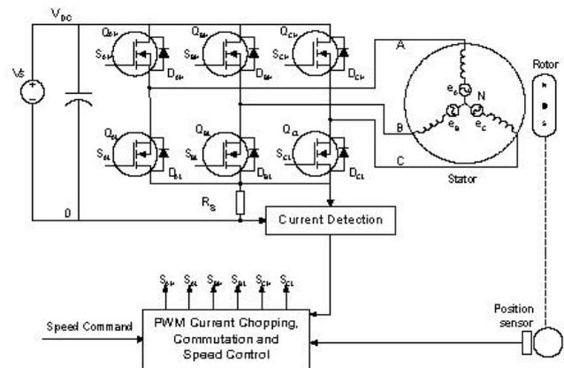
Fig. 3. Schematic of a spindle motor system with rotor position sensors.
