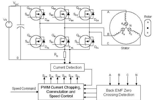
Fig. 6. Schematic of a sensorless spindle motor system.
