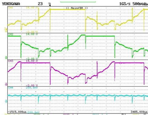
Fig. 4. Waveforms of terminal voltages and DC link current of a typical HDD spindle motor in MOESFET on-resistance control mode.
