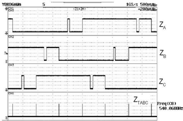
Fig. 16. Phase back EMF ZCP pulse signals.
