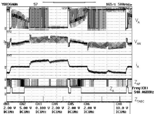
Fig. 17. Typical voltage and ZCP signal waveforms of phase A.
