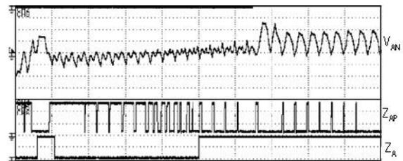
Fig. 14. Phase *A* voltage ZCP signal without PWM chopping noises.
