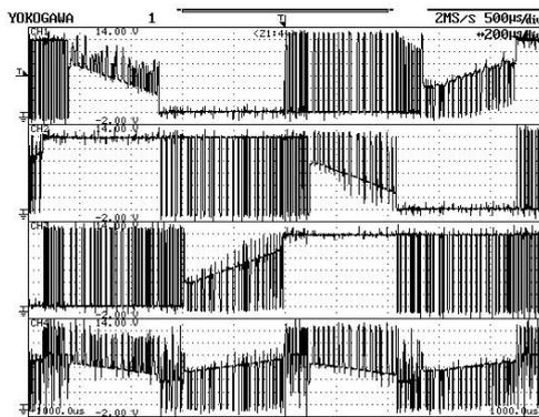
Fig. 5. Waveforms of terminal voltages and neutral voltage of a typical HDD spindle motor in PWM chopping control mode.
