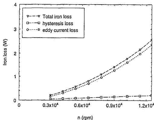
Fig. 1 Iron loss in 8-pole 9-slot spindle motor
