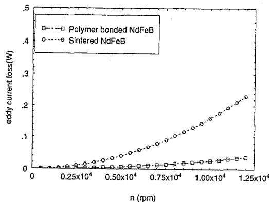
Fig. 5 Predicted eddy current loss in rotor
