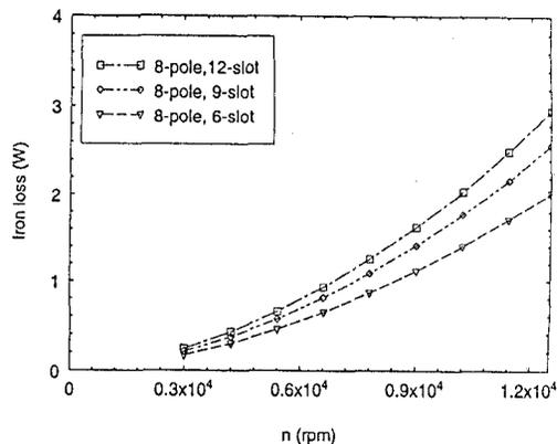
Fig. 2 Iron loss in Motor A, Motor B, and Motor C
