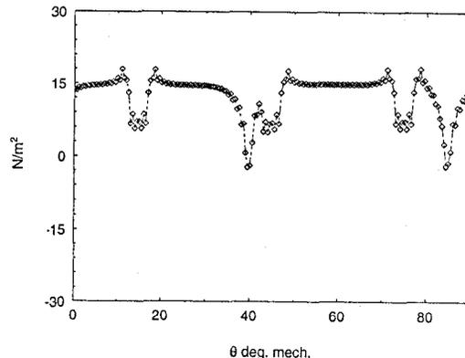
Fig. 4 Maxwell tensor vs.  $\theta$  for Motor C
