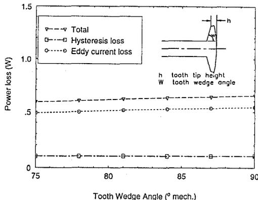
Fig. 3 Effect of wedge angle on iron loss in Motor C at 5400 rpm
