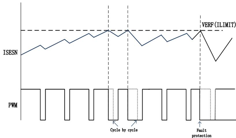
Figure 3 Cycle by cycle current protection mode
